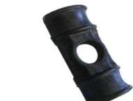
奔驰 钢板盖板 73510126/001 Benz Spring seat plate
