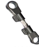
扭力杆 BPW Adjustable Rod Arm
