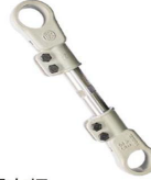
扭力杆 BPW Adjustable Rod Arm
